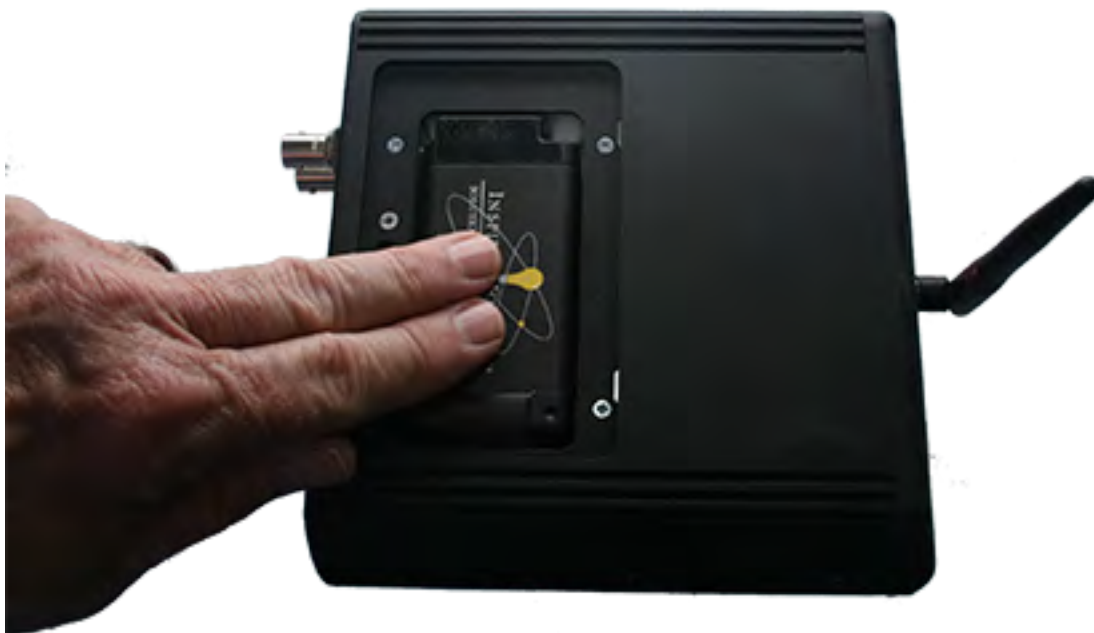
Figure 2.7 - Sodera Battery: Press to Make Contact
