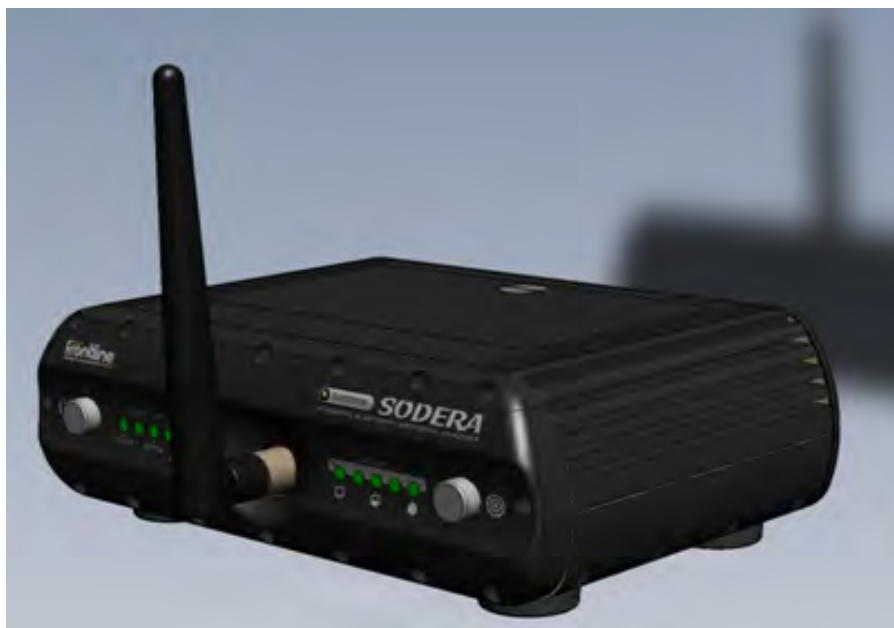
Figure 2.3 - Antenna Attachment Point
