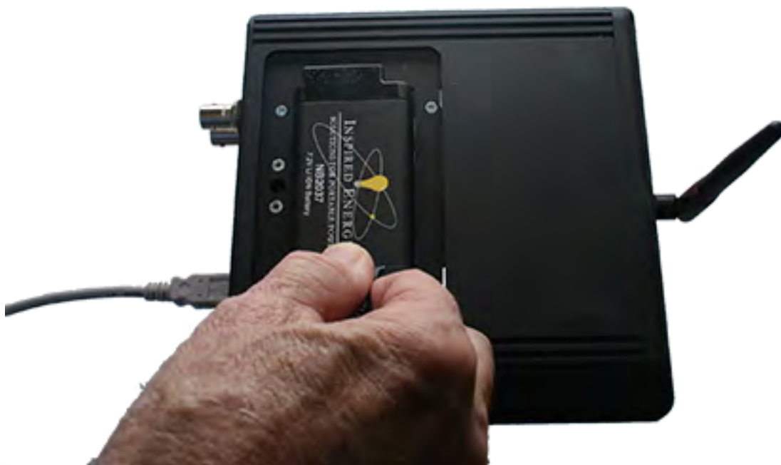
Figure 2.5 - Sodera Battery Removal Using the Tab
