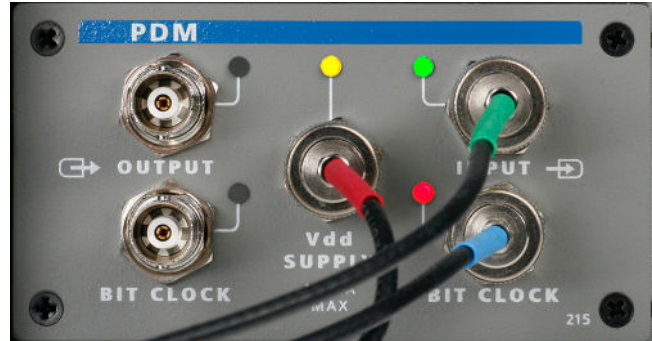
Figure 6: APx PDM module, connecting the output of a PDM MEMS microphone to the PDM input on the APx analyzer.
