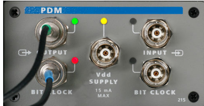
Figure 11: APx PDM module, connecting the APx PDM output to the PDM input on a device.
