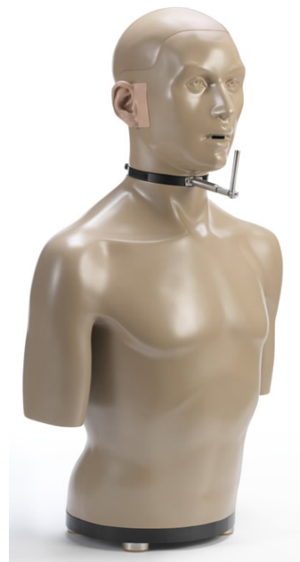
Figure 7: KEMAR 45MB HATS manikin with mouth simulator.
