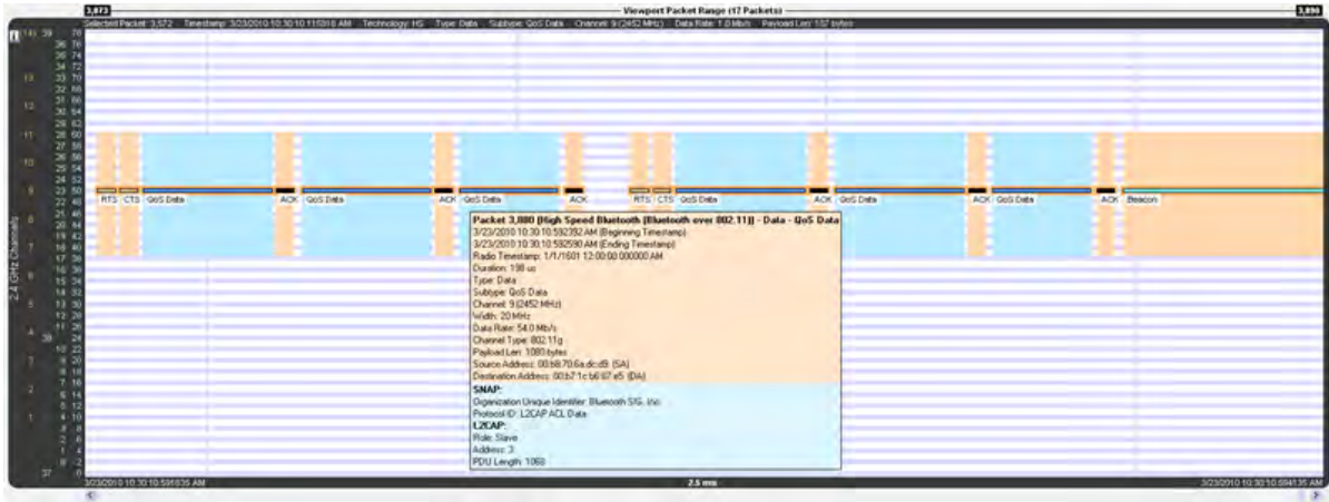
Figure 4.79 - High-speed Bluetooth packets have a blue frequency box and a two-tone tool tip
