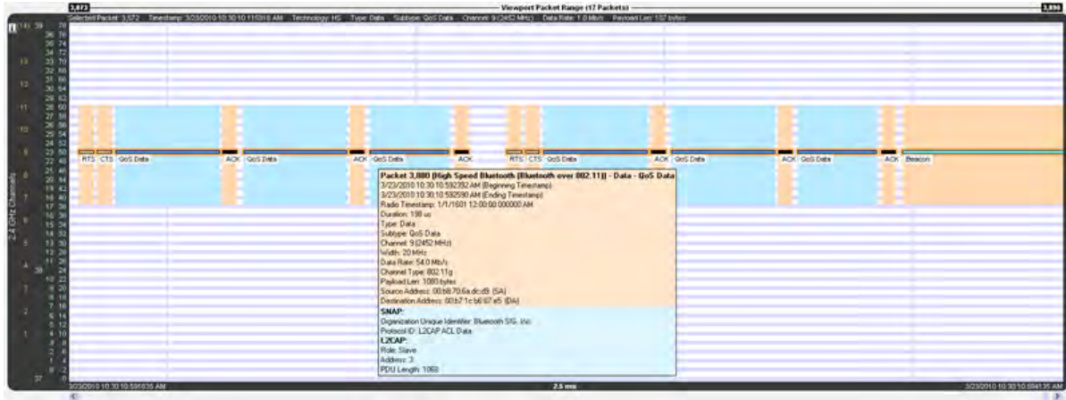
Figure 4.97 - High-speed Bluetooth packets have a blue frequency box and a two-tone tool tip
