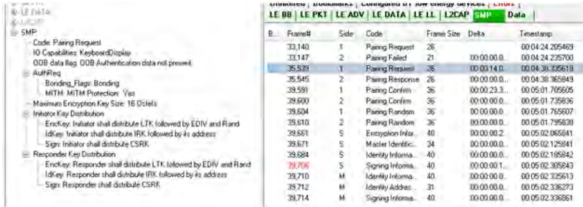
Figure 23 - SMP Pairing Request (Frame# 35,539) from Initiator (Side 1)
