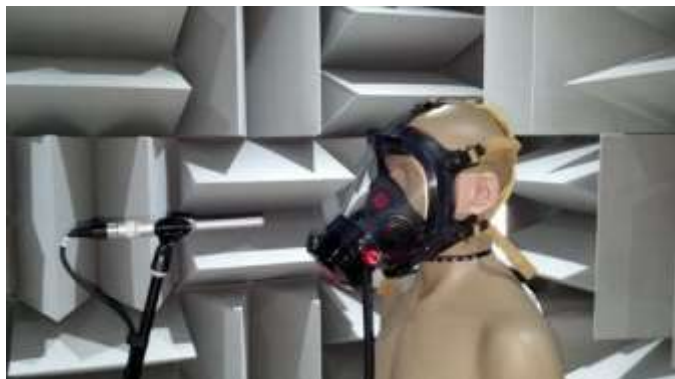
Figure 7. 無響室でSCBAを装着したGRAS社製KEMARマネキ [Photo courtesy of Scott Safety, used by permission.]
