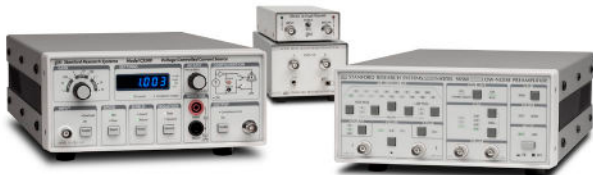
SRS current source and several SRS preamplifiers
