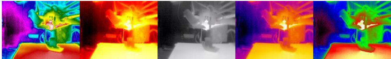
Sample Lepton 3.5 thermal images showing a finished 3D printed object imaged with different colorization settings.
