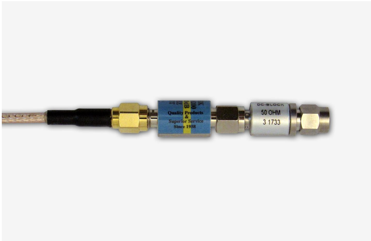
Figure 2.3 – DC Blocker Connection to Attenuator
