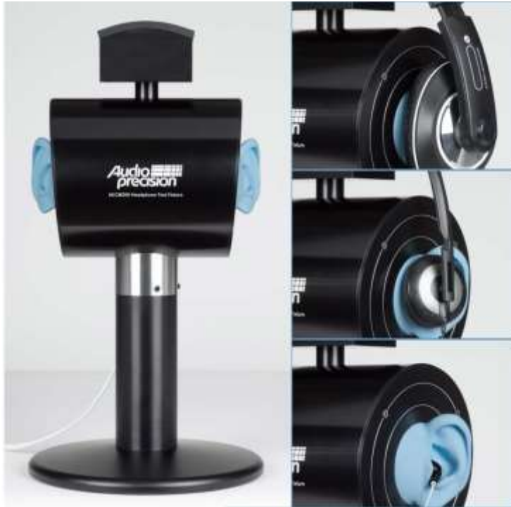
Figure 6. Audio Precision AECM206 headphone test fixture.
