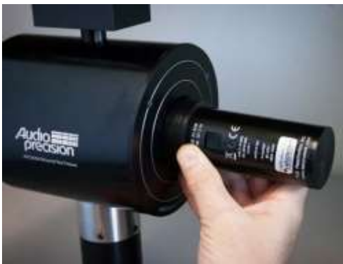
Figure 11. Using a CAL250 sound level calibrator to calibrate a test fixture's ear simulator microphone.
