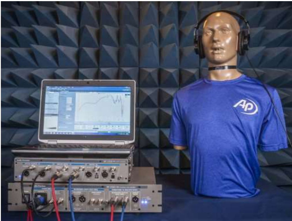
Figure 5. An example of a Head and Torso Simulator called KEMAR, made by G.R.A.S Sound and Vibration.
