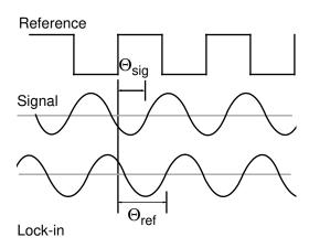
The lock-in amplifies the signal and then multiplies it by the lock-in reference using a phase-sensitive detector or multiplier. The output of the PSD is simply the product of two sine waves.
