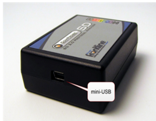
SD 2.0 Hardware Interface - Analysis Side Showing USB mini-B Receptacle
