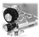
Weinschel's 940 series uses a card resistor on a disk with a movable coaxial contact (shown below) similar in nature to a potentiometer and provides an incremental range of 114 dB incremental range at 2 GHz and 60 dB at 4 GHz. Because the shunt film is connected to ground permanently, in order to achieve the extended attenuation range, the minimum loss of this type attenuator is higher (4 to 6 dB).
