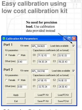
Reference plane offset and open circuit capacitance coefficients allow a **tailor-made kit** to be built
