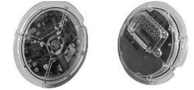
Electronic Safety, Arming and Initiation Device (ESAID) for ground to air missile application
