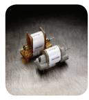
An open frame RF reed relay with 8kV isolation and 6A (at 30MHz) carry current, the FRD12000 series has been used many HF radio system specifications over the years, with applications in commercial maritime (GMDSS) equipment and military HF radio units worldwide. The use of vacuum reed switches with rhodium contacts offers high isolation voltages, low contact resistance and long operating lifetime.
