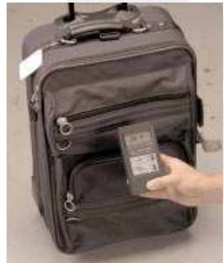
palmRAD 907 shown above. Used to locate radiation and measure in \mu R.
